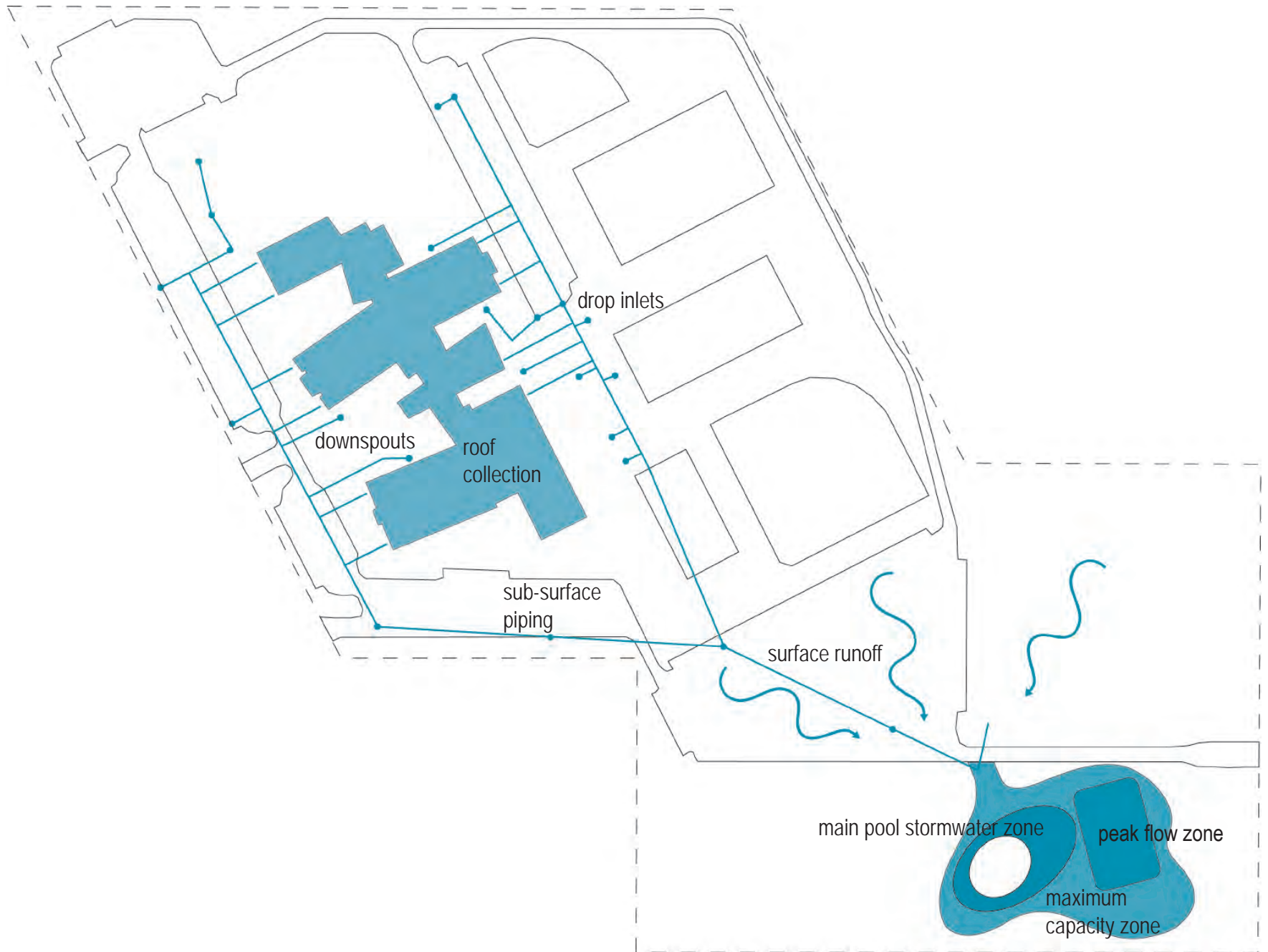
Figure 37 Stormwater collection system.
