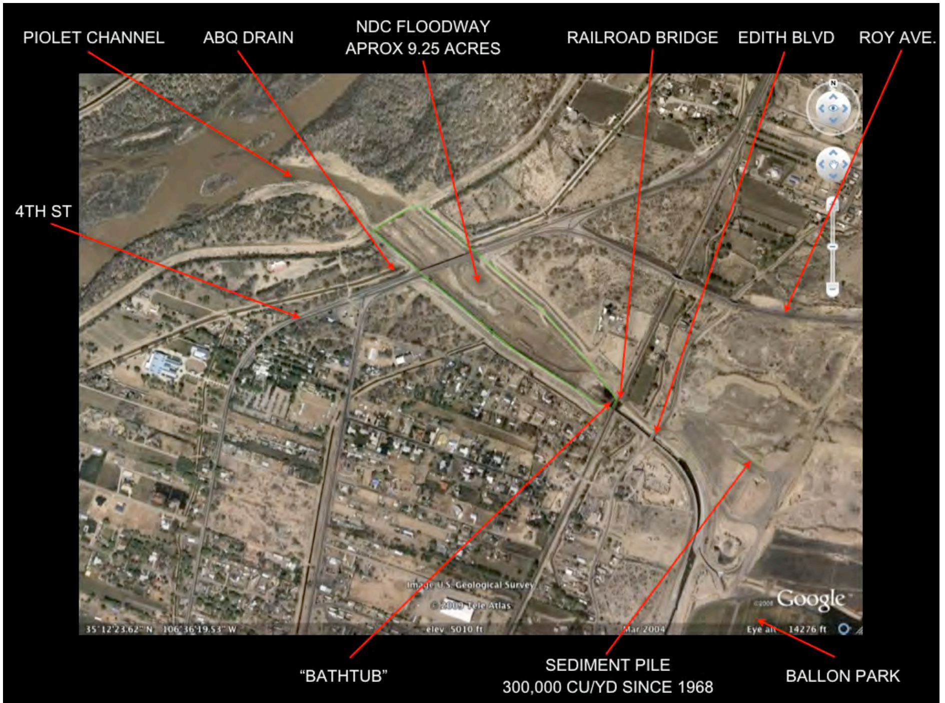
North Diversion Channel outfall component locations.
