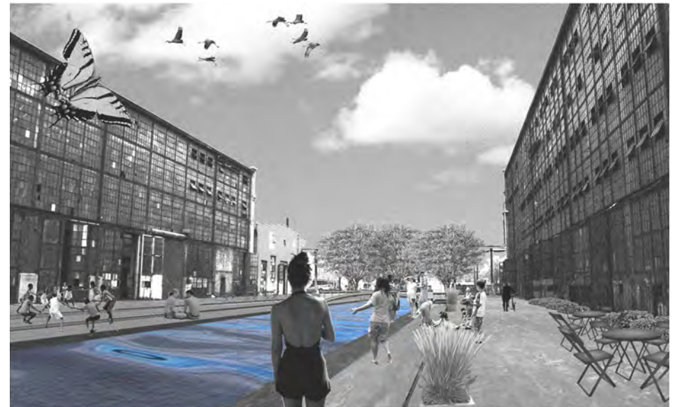
Figure 34. The reflection pool is where stormwater is stored after it has flowed through the constructed wetland and prior to being used for irrigation. This storage infrastructure doubles as a reflection pool, providing a unique urban environment cooled by the shade of industrial buildings and the presence of water. Image from the author.
