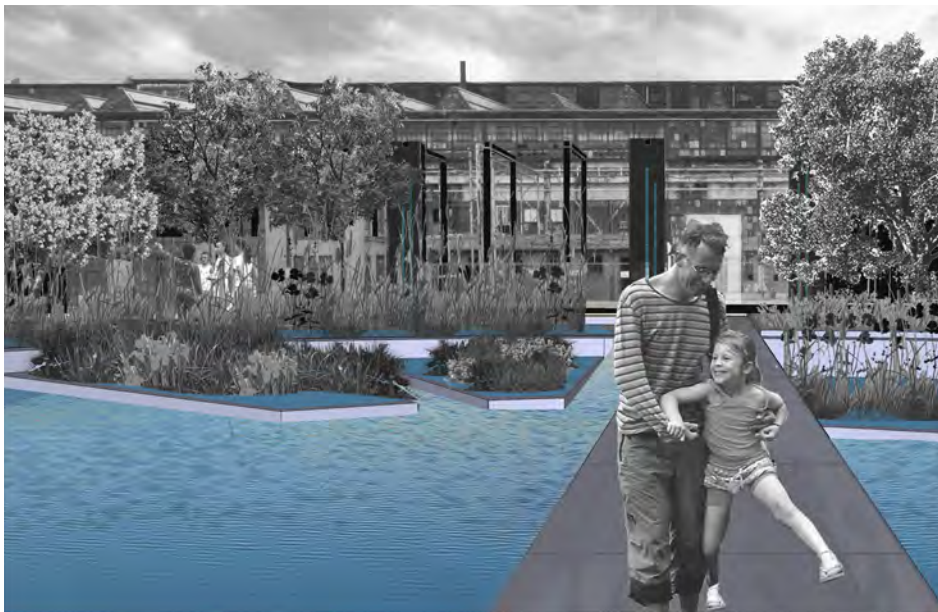
Figure 32. A bridge crosses all terraces of the constructed wetland, remaining level with the surrounding finish floor elevation. Stormwater flows through a series of 1' deep terraces full of wetland plants that have the ability to remove pollutants from the water. The deep center pool stores water after it has been remediated and before it flows into the reflection pool to ultimately be used for irrigation. Image from the author.
