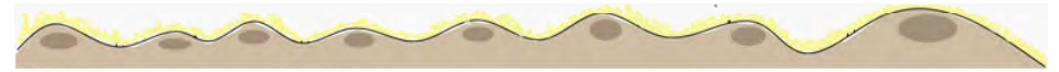
Figure 24. Linear mounds of contaminated soil will be formed in the fields (southern) portion of the design and will be inoculated with oyster mushroom mycorrhiza and planted with Indian mustard to remove lead and hydrocarbons from the soil. Image from the author.
