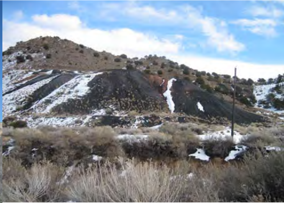
Fig. 26: Typical gob piles along the arroyo in Madrid. The piles' erosive qualities are visible in this image.
