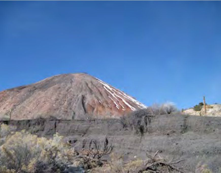
Fig. 25: Red Dog, or 'clinker' gob piles along the arroyo in Madrid; red dog piles are gob piles which have caught on fire through spontaneous combustion.
